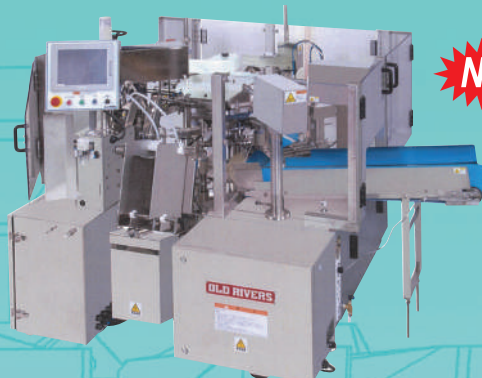
▲ FF-220NIII 日本古川全自動取袋充填封口包裝機 Vertical Type Computer Touch Controlling Auto Filling-Sealing Machine
